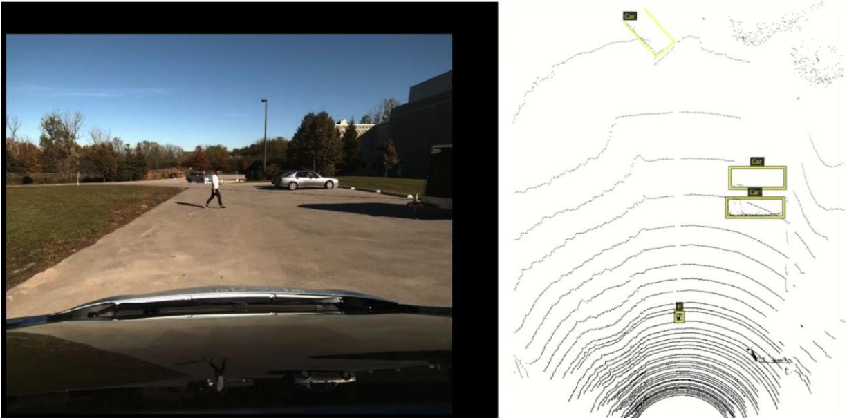
Figure 4. Labeling interface with camera view on the left and BEV of pointcloud with labelled objects on the right.
